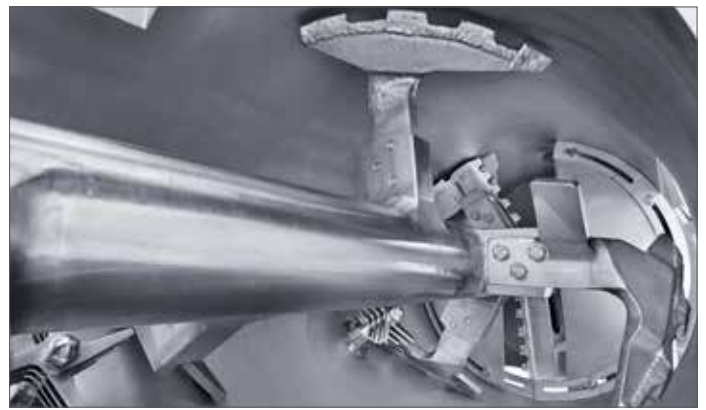
View inside mixing drum
