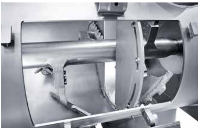
Opening in the drum with overflow weir arranged in front of it
