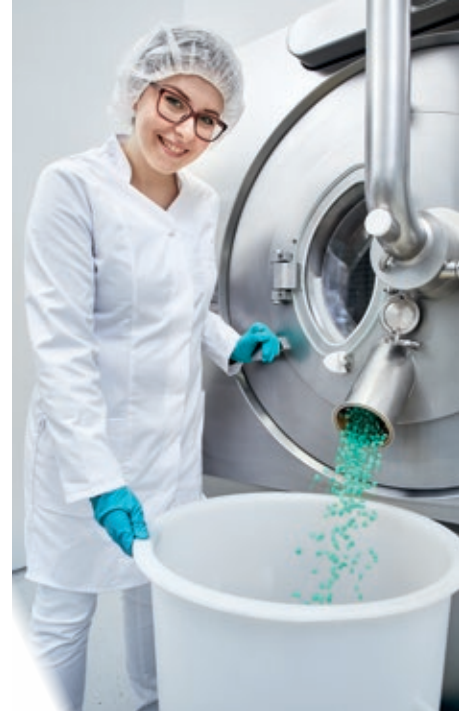
Coater discharge through the outlet at the front of the coater
