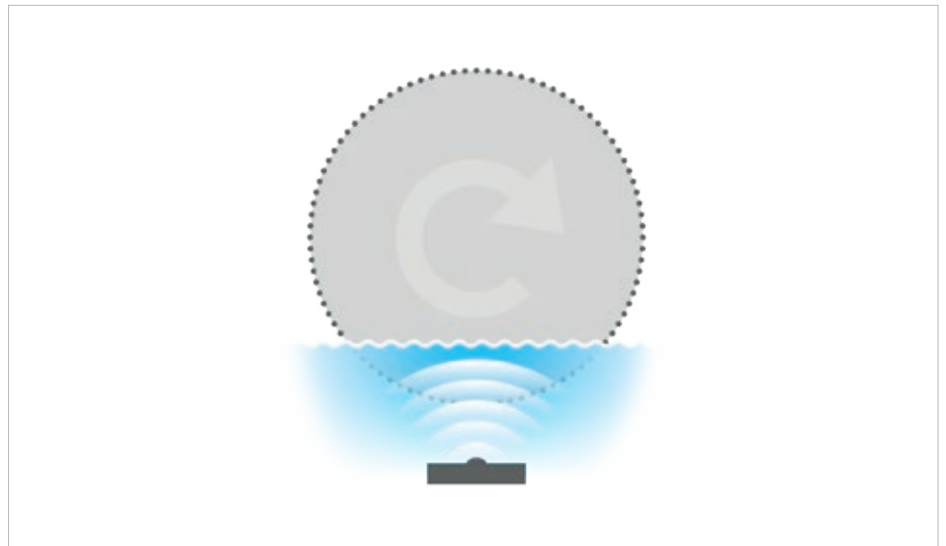
To speed up cleaning of the drum perforation, an ultrasound generator can be integrated in the cleaning system of the LC series*.
